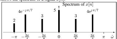
(a) [10] Determine the N-point DFT coefficients X[k] of this signal, where N is the fundamental period of x[n]. Your answer should be a formula or a list in the form
