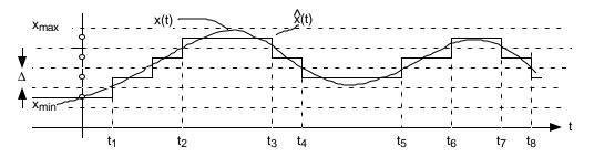
Observation: When  $\Delta$  is small, x(t) is approximately a straightline in most of the time intervals where the output  $\hat{x}(t)$  is constant.
