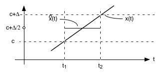
The straightline has an equation: x(t) = at + b, where  $x(t_1) = c$ ,  $x(t_2) = c + \Delta$ , and  $a = slope = \Delta/(t_2-t_1)$ . Let us now find the MSE in the time interval [t<sub>1</sub>,t<sub>2</sub>]:
