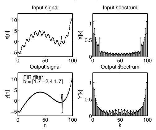
So this FIR filter appears to remove 60Hz hum pretty well. Where did the coefficients, the  $b_k$ 's, come from? This is the subject of filter design, which we will tackle in Chapter 7.
