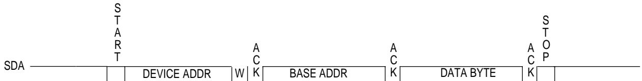
Figure 16-126. Byte Write to Device with Internal Addresses
