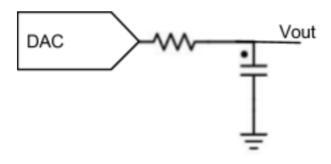
$$R_f + R_{adc} = 1/(C2\pi f)$$
