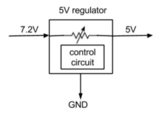
Power dissipated thru regulator is P=IV where V is voltage drop across regulator  $P=(7.2\,V$  -  $5\,V)$  \*  $200\,mA=440\,mW$
