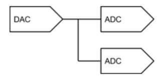
If voltage is half,  $R_{adc1} \parallel R_{adc2} = R_{dac}$  to satisfy voltage divider rule So  $10 \,\mathrm{k}\Omega = 20 \,\mathrm{k}\Omega \parallel 20 \,\mathrm{k}\Omega$
