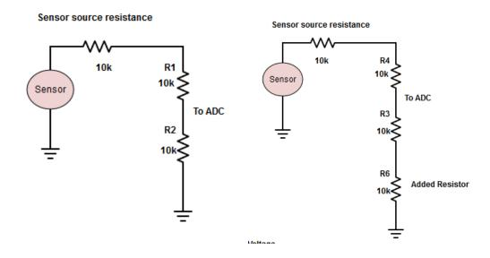
The second possibility is the input of the ADC resistance is 10K and the sensor source resistance is very low. Then the voltage provided to the ADC is
