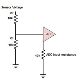
To fix it, put a 10k in parallel with R9 to balance the divider.
