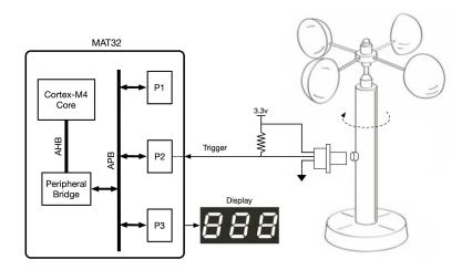
This fictional MCU has the following APB3 bus interface. The ABP bus signals follow APB timing and protocol. Read and write cycles are provided on the next page. PSEL is configured to be "1" when memory locations **0x40050000-0x40050007** are accessed.
