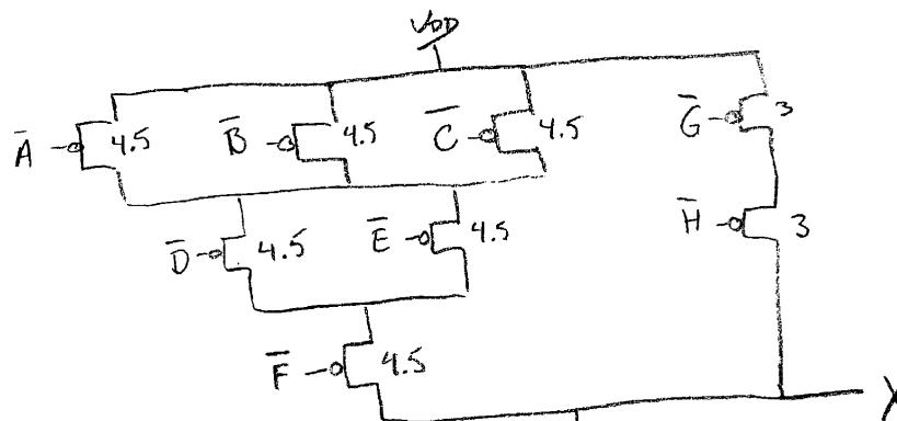
Numbers are transistor widths, in microns.
