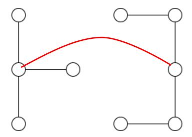
a. As a NoC topology designer, what *single link* would you add between *any two processors* in this network to minimize the average hop distance in the NoC? Draw the link above and give a one-sentence explanation. (Note: the length of each link is not a consideration for this question.)
