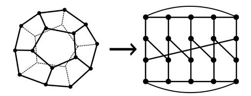
A dodecahedron is a polyhedron (three-dimensional polygon) with twelve faces, wherein each face forms a regular pentagon. The left figure shows a 3D dodecahedron as seen from above, dotted lines indicating edges on the hidden faces. A router can be placed at each of the 20 vertices of the shape. The right figure illustrates an equivalent planar topology—how the topology can be laid out in a regular grid on a 2D plane. This is how an actual chip using such a topology would be connected.
