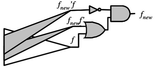
figure 6: Resynthesized next-state function
