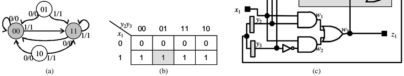
Figure 2: (a) The modified STG of the retimed circuit of Fig. 1(b), (b) the karnaugh map of the next-state function of  $y_2$  (the next-state function of  $y_3$  is identical), and (c) the resynthesized circuit that preserves the set of synchronizing sequences
