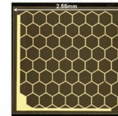
Microscope image of II-VI ZnTe:O intermediate band solar cell.
