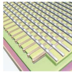
High-density memory and logic circuits can be utilized using the memristor-based crossbar circuit illustrated above.
