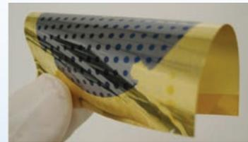
Epitaxial lift-off allows for the transfer of thin mat-III-V layers onto flexible substrates. An array of InP-Indium tin oxide is shown mounted on a Kapton substrate.
