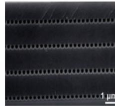
4 levels of 200nm-wide nanochannels formed by reversal nanoimprint in SU-8.
