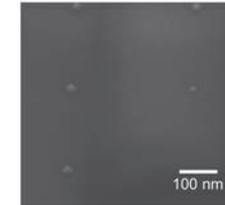
Site-controlled InGaN/GaN quantum dots for single-photon emission.
