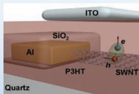
Single-walled carbon nanotube high-efficiency hybrid photovoltaics.
