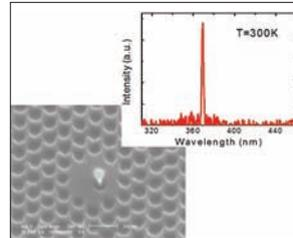
Single GaN nanowire laser on silicon with photonic crystal cavity.
