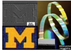
High-efficiency, high-resolution plasmonic color filters using nanostructured metal-dielectric-metal stacks (left). Nanogratings on a flexible substrate fabricated by high-speed and continuous roll-to-roll Nanoimprint process.
