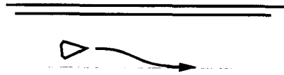
Fig. 18. Defining closed-loop path-following behaviors. The learning agent uses the dynamic action model to add error correction to an open-loop path-following behavior in order to obtain a closed-loop path-following behavior. In this example, a small turning motion is used to keep the robot on the path as it advances.
