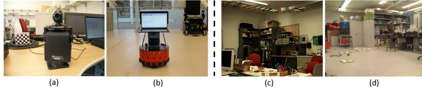
Fig. 2. (a) A webcam on a pan tilt unit, (b) A webcam on a mobile robot (the webcam is a built-in device at the center of the top edge of the laptop monitor), (c)-(d) Off-line learning environments for the two robots respectively.
