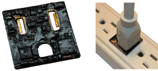
Figure 16: Conformally coated PowerBlade. Shown are the unit after conformal coating has been applied, as well as the conformally coated unit attached to a load. Although this method requires a manual application process that is not manufacturable in large scale, it does protect the user from live parts. In the future an overmolding process will provide similar protection in a manufacturable way.
