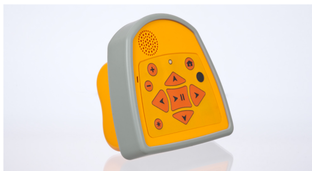
Figure 1: The Talking Book: a state-of-the-art rural audio computer designed specifically for on-demand information access in developing regions. To access audio content, users navigate through voice prompts using the small number of orange input buttons visible on the device.
